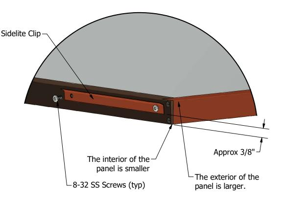
Note: Sidelite Panels have tapered edges. The larger side faces outward.
