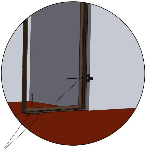
Drill and countersink for screws, shim as needed (typ)
