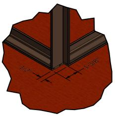
4. Replace front frame and attach frames and cornerpost together with machine screws
