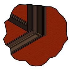
3. Remove front frame, position cornerpost and fasten toe screws
